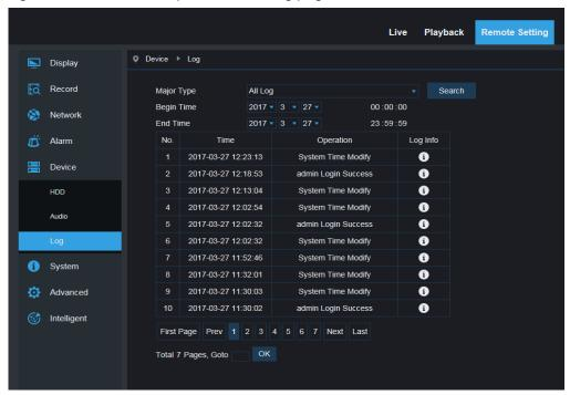
Log Type: Eight types of logs are available - system logs, network logs, parameter logs, alarm logs, user logs, recording logs, storage logs and all logs). Choose the starting and ending date/time for retrieval.
