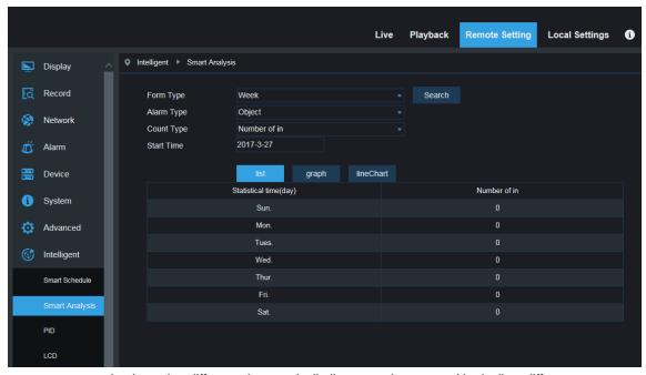
This page can correctly show the different time period's line crossing count (including different years, months and weeks' line crossing count). User can search the video according to the recording types, alarm types and the beginning time of the recording.
