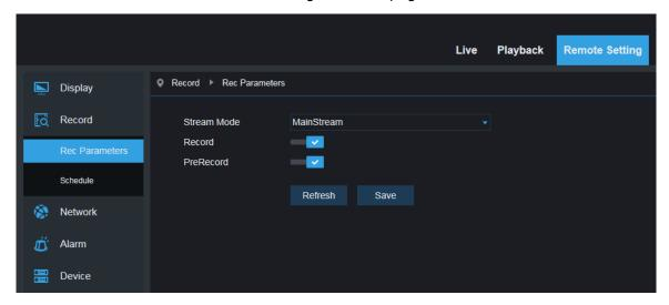
This function is to control the record, pre record and record type (main stream and substream)
