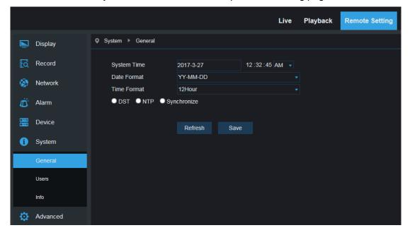
The device time, system time, date format and time format contained in the basic information can be manually set and saved.
