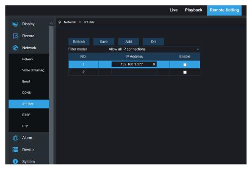
**Filtering mode:** Three modes are available (Allow all IP connections, Allow all IP connections as set, Forbid IP connection as set).
