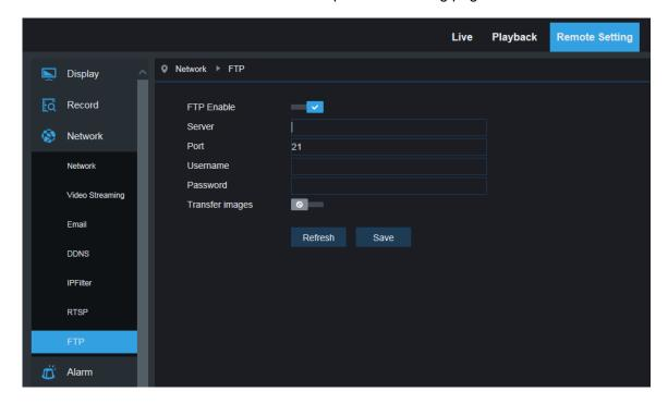
**FTP**: FTP service setting - used with alarm function to upload images or videos snapped to the FTP server.
