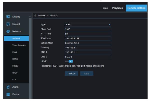
Networking mode: DHCP (Automatically Acquired), Manually Configured and PPPOE; the default is
