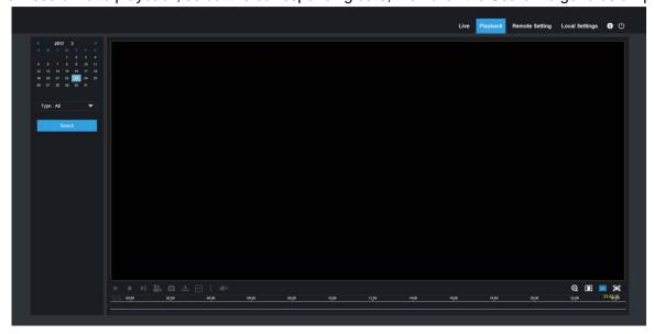
User can search video by file type as needed, and operate the video through the simple tool on the toolbar, e.g. open/stop video , bit stream video, recording, snapshot, download recording , quick motion video playback, Sound On/Off.
