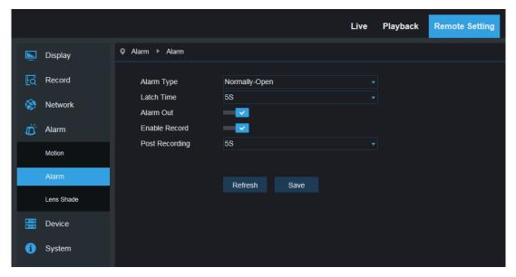
I/O Alarm Input: Enable or disable I/O alarm.
