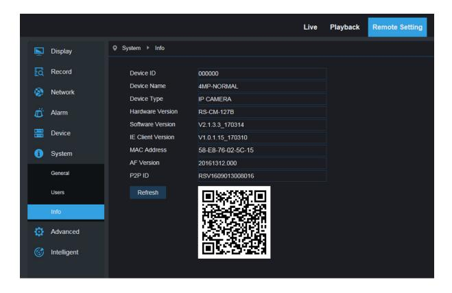
Here some system information on the device will be displayed, including device type, MAC address and software version.
