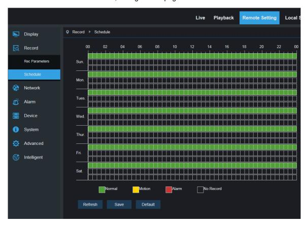
As image: one grid in the table is 30 minutes, green is normal record, yellow is motion detection alarm, red is I/0 User can setup according to private requirement to choose different record type and time.
