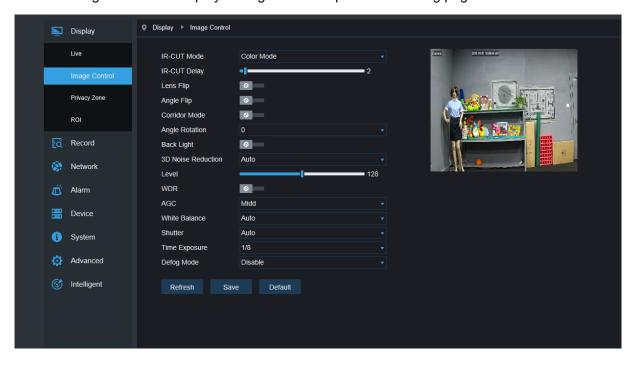
IR-Cut Model: Classified into GPIO Automatic, Colored, and Black-White models.
