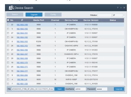
Config: Double-click the selected camera in the search page, turn to the Config page to reboot the camera, change passwords, and reset the camera.
