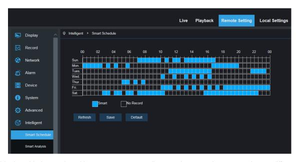
one grid in the table is 30 minute,User can setup according to private requirement to choose different record type and time  $_{\circ}$
