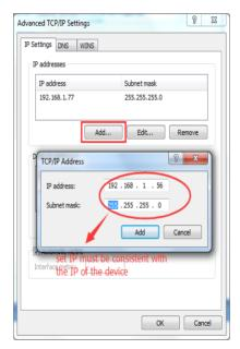
Note: When software IPC Device Search is used for search, which employs multicast protocol to search network information on the equipment across segments, and no multicast data packet is permitted by any firewall, so a firewall must be disabled to acquire network information on the equipment. Step 2: Run the IP search tool Device Search provided in the CD as attached.
