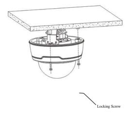
Fix the front component on the pedestal by tightening the three locking screws.
