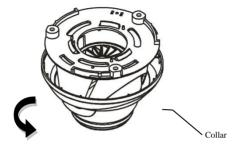
Remove the collar off the camera by rotating it down
