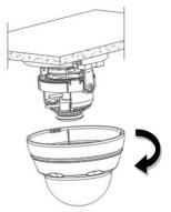
After angle adjustment, mount the shield back by rotating the collar up.
