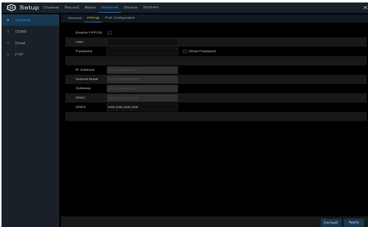
This is an advanced protocol that allows the NVR to connect to the network more directly via DSL modem.
