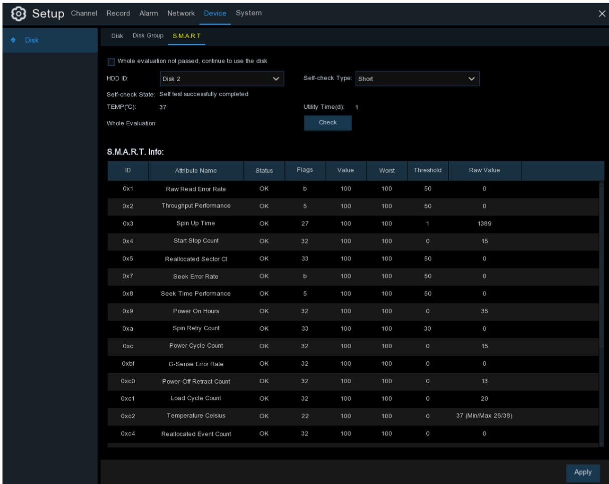
**Whole Evaluation not passed, continue to use the disk:** If for some reason the hard drive has developed a fault (such as one or more bad sectors), you can instruct your NVR to continue saving to the drive.
