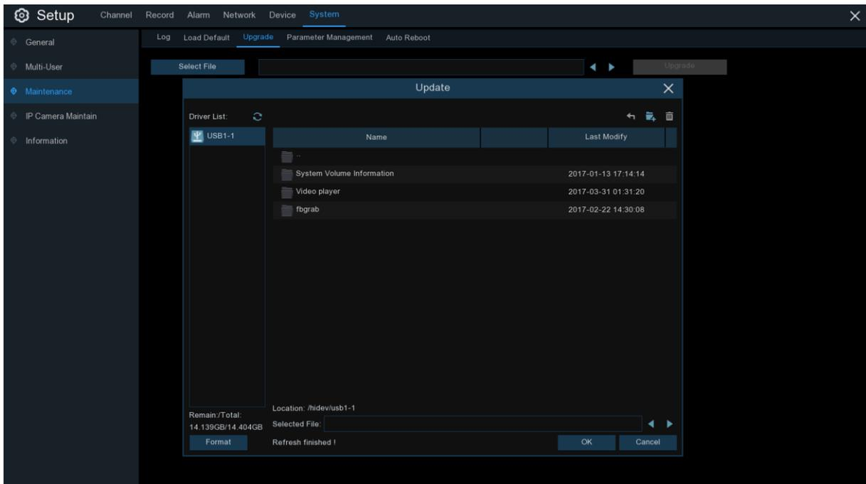
1. Copy the firmware file (.sw file) to your USB drive, and insert the USB flash drive into the NVR's USB port.
